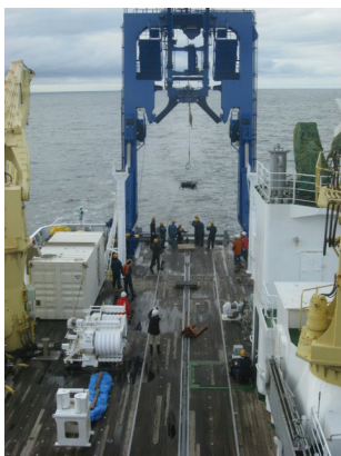
Ship's crew and science crew trial rig science packages on stern mounted 22 ton A-Frame for upcoming science station
